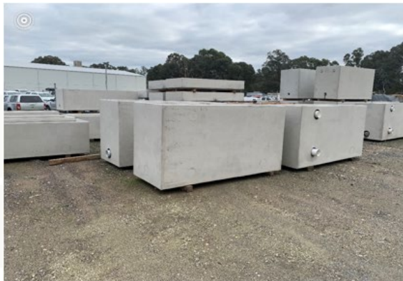
Some finished raw concrete tanks
