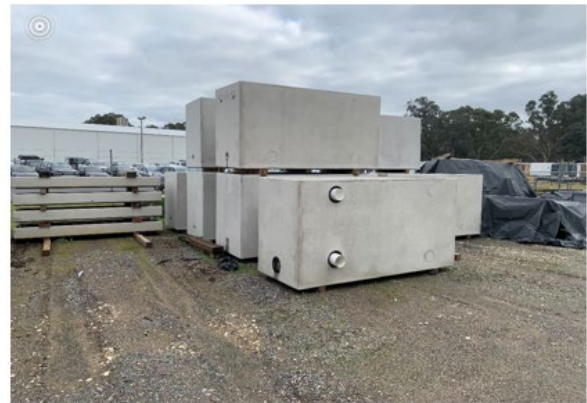
Some finished raw concrete tanks stacked next to tank lids
